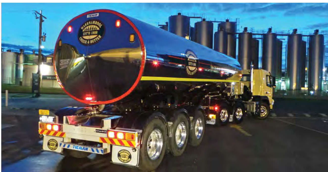
WCB was the first Australian company to fit tankers with these reflective strips for safety (Photo by Tieman). Photo opposite by B Elton.
