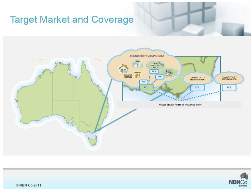
Figure 3.1 NBN Co Access Architecture
