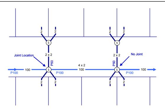
A conservative view would see the pits on the opposite side of the street to the distribution cables omitted in 75% of cases. In these cases, the lead-in conduits can be extended in a protective "enveloper" conduit under the road to the pit on the opposite side of the street.
