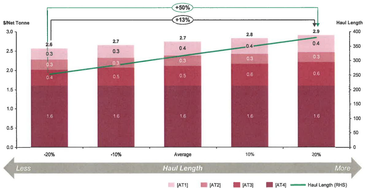
Figure 6 – Illustrative Below Rail Cost per Net Tonne by Indicative Haul Length, Blackwater System
