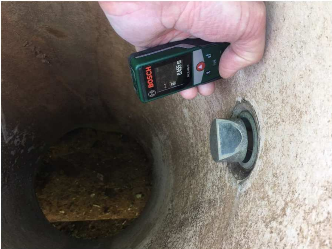
Figure 5. A used James Hardie 450 mm nominal diameter pipe being measured. The MACE Doppler sensor is shown.
