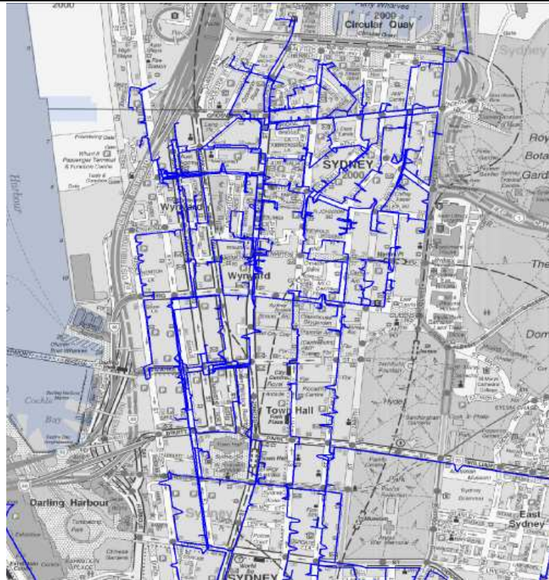
Figure 4: Optical fibre loop deployment by Powertel in Sydney
