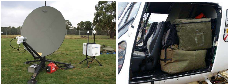
Fly-away Satellite Cell on Wheels (SatCOW) – both set up and ready for transport by helicopter
